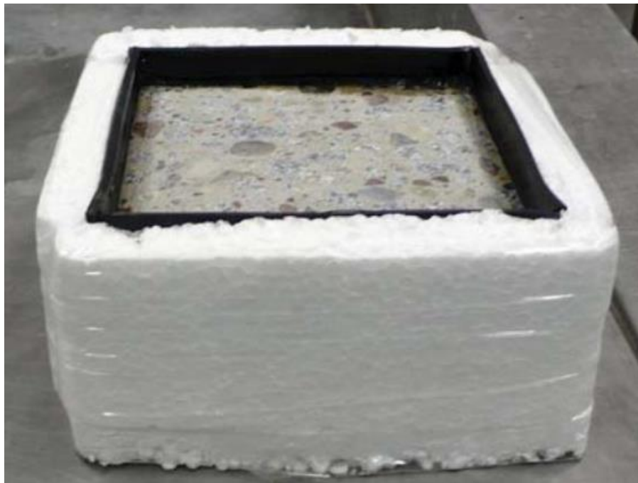
Figure 4. Prepared sample before Slab Test - Freeze/Thaw Resistance of Roller Compacted Concrete.
